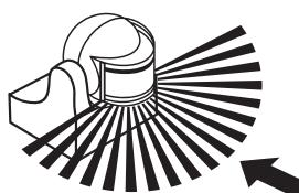
incorrect direction of movement / helytelen mozgásirány /
